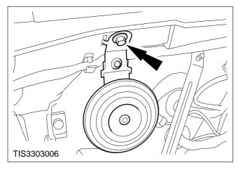
3. Remove the alarm horn.
