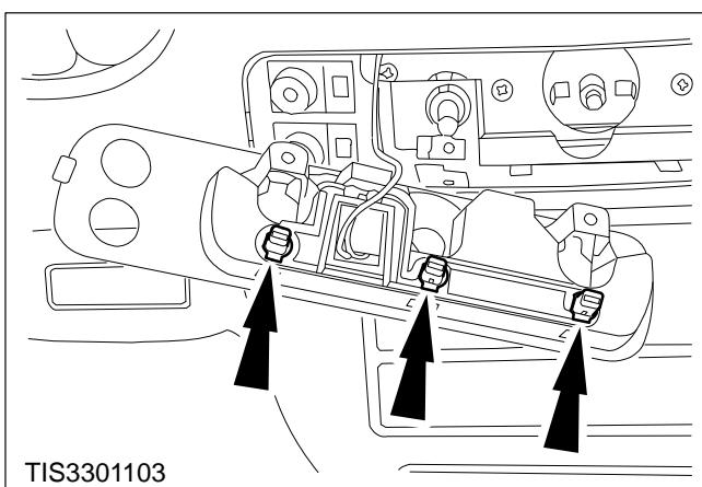
**Bulb – Heater Control Illuminating – Remove (33 128 0)**
