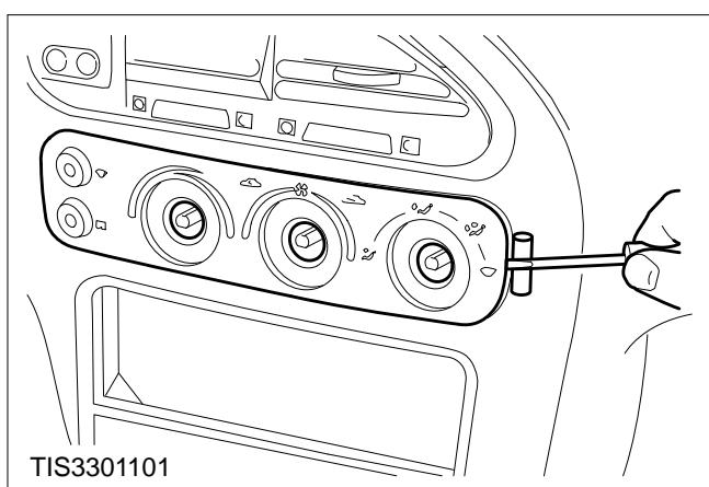
**CAUTION:** Only prise out the bezel from the air distribution control switch side of the bezel to prevent breakage of the locating tang at the opposite side.
