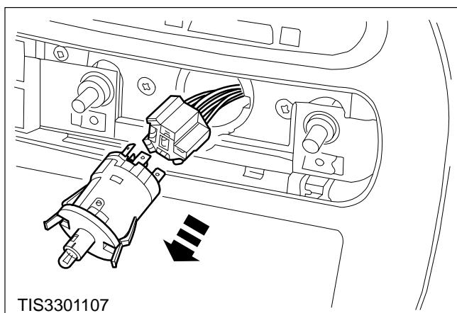
11. Disconnect the multiplug and remove the switch.
