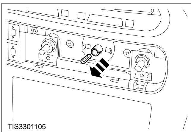
**Bulb – Heater Motor Switch – Remove (33 120 0)**
