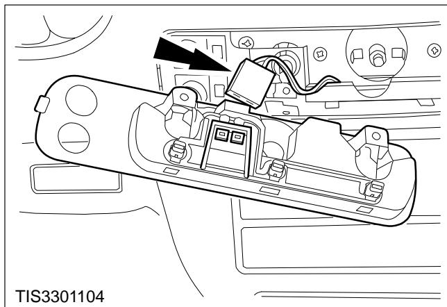
9. Disconnect the multiplug and remove the heater control bezel.
