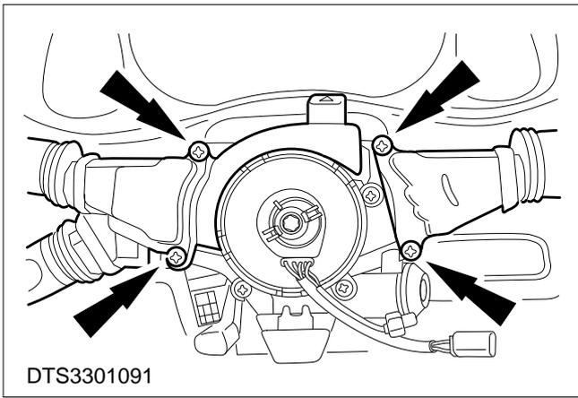
**4. Detach the appropriate switch (two screws).**
