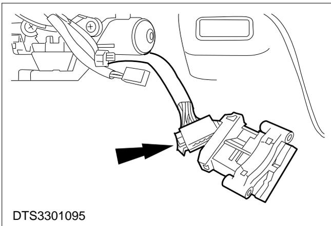
**5. Disconnect the multiplug and remove the multifunction switch assembly (right-hand multifunction switch assembly shown).**
