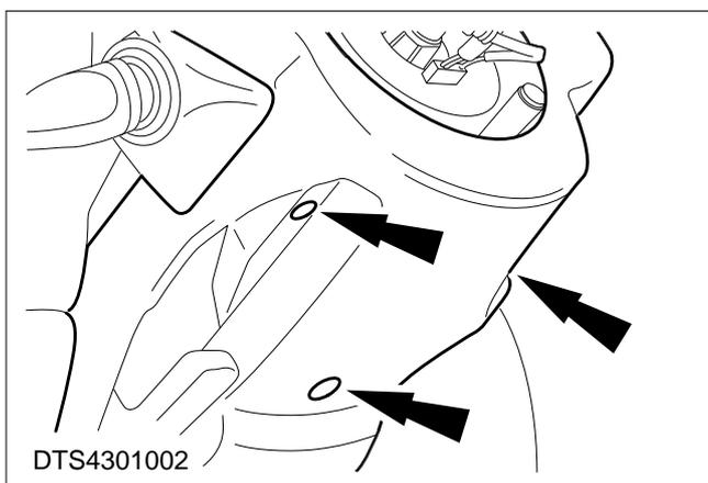
3. Remove the lower steering column shroud (three screws).
