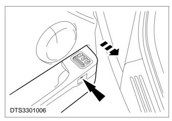
2. Loosen the retaining screw and pull the door pocket forwards.
