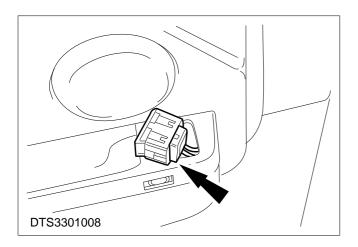
4. Disconnect the multiplug and remove the switch.
