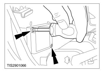
5. Unscrew the retaining bolts and remove the El system module.
