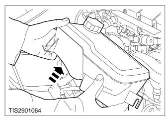
3. Carefully lift the degas tank to one side.
