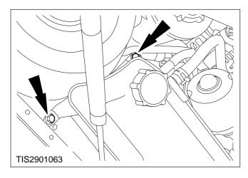
2. Unscrew the degas tank retaining bolts.
