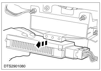
7. Remove the PCM from the bracket.
