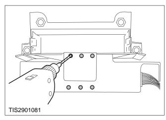
CAUTION: Do not allow the drill to make contact with the PCM casing.
