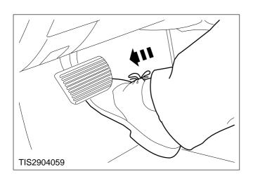
12. Depress the accelerator pedal fully and release slowly.
