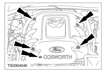
7. Unscrew the nuts and remove the engine cover (V6 24V variants only).
