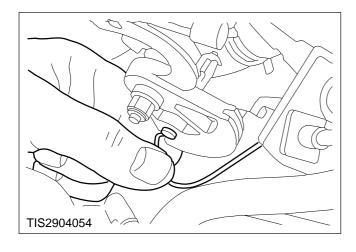
11. Reconnect the inner cable to the throttle body.
