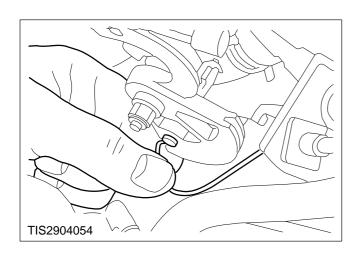
8. Disconnect the inner cable from the throttle body.
