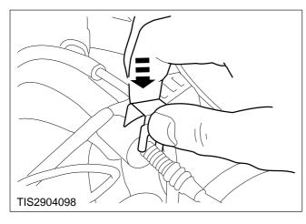
13. Refit the clip to the TCS motor/throttle body cable adjuster.
