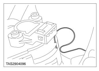
6. Insert the TCS motor lock pin through the pulley alignment holes.
