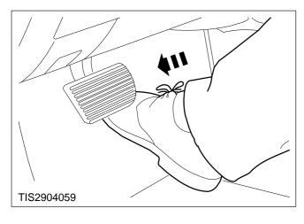
9. Depress the accelerator pedal fully and release slowly.
