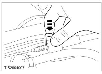
10. Refit the clip to the accelerator pedal/TCS motor cable adjuster.
