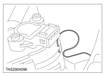
14. Remove the TCS motor lock pin.
