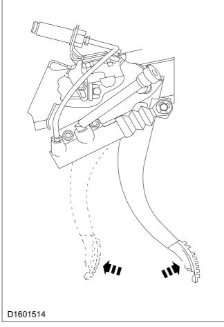
**NOTE:** The pedal travel must be limited by the master cylinder and not by switches or insulating matting.
