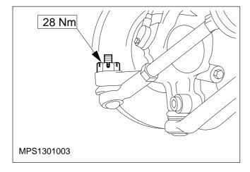
7. Refit the track rod end ball joint to the spindle carrier and secure the castellated nut with a new split pin.
