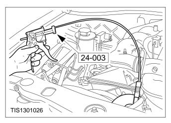
8. Remove the cooling system top hose.
