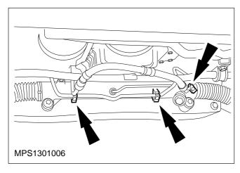
15. Disconnect the power steering pipes from the steering gear.
