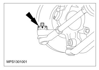
6. Remove the split pin and castellated nut from the steering track rod end.
