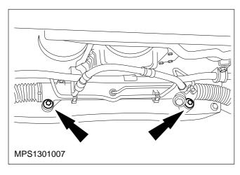
10. Remove the steering gear.
