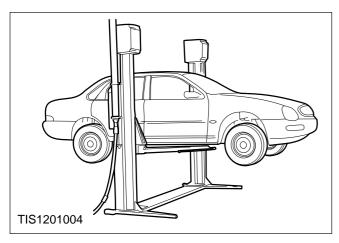
3. Slacken the wheel nuts, raise the vehicle and remove the front road wheels.
