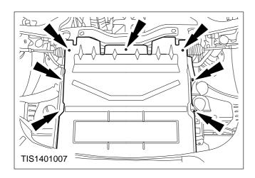
4. Remove the lower engine shield.
