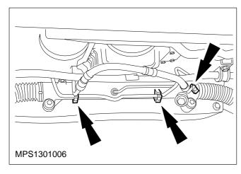
9. Disconnect the power steering pipes from the steering gear.
