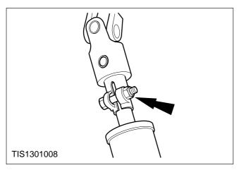
11. Remove the flexible coupling from the steering gear pinion.
