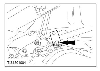
5. Remove the clamp plate bolt securing the flexible coupling to the steering column shaft.
