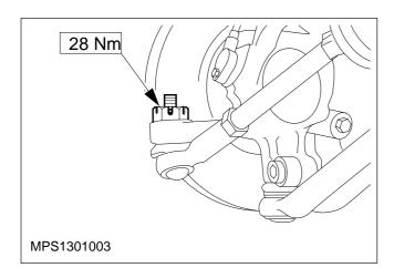
16. Refit the track rod end ball joints to the spindle carriers and secure the castellated nuts with new split pins.
