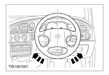
1. Centralise the steering wheel and lock in position.
