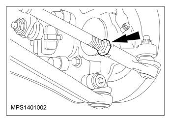
2. Slacken both the track rod end locknuts.
