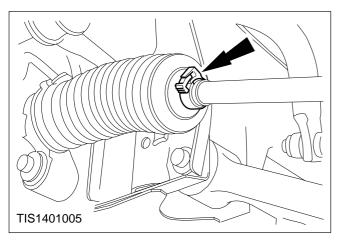
3. Remove the bellows outer retaining clips.
