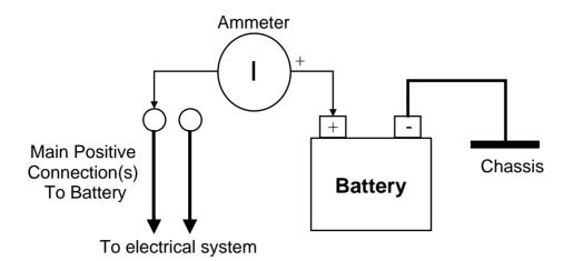
If the current flowing is over 80mA a problem exists with a discharge fault someplace in the electrical system. This must be found and rectified. A faulty Alternator short circuited Diode can also cause this problem. After factory equipment, Car Cell phones, Alarms etc can often add excessive discharge currents.
