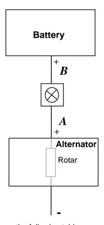
This can provide useful information on the health of the system, the following table may help when fault finding the Scorpios charging system. Note the Warning Light may not show subtle faults, also if the regulator or diodes are open circuit the light will not illuminate
