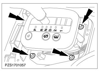
9. Remove the selector lever assembly.
