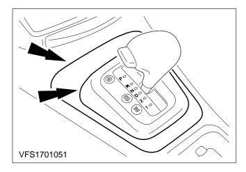
23. Install the bezel and cover of the selector lever assembly.
