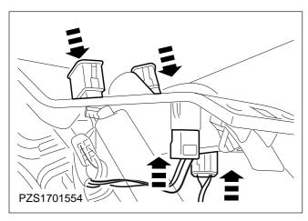
18. Connect the plugs and fit the two switches.
