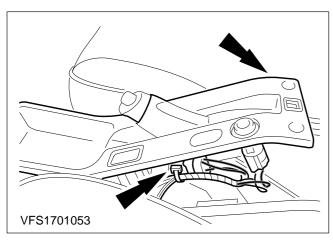
4. Lift the switch console over the handbrake lever and cut the cable ties.
