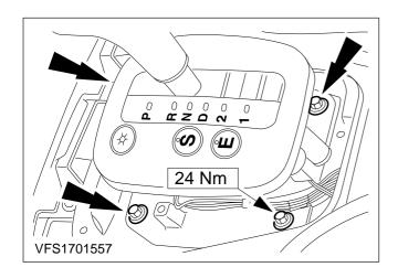
14. Install the selector lever assembly.
