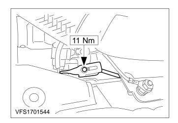
6. Tighten the selector rod clamp bolt.
