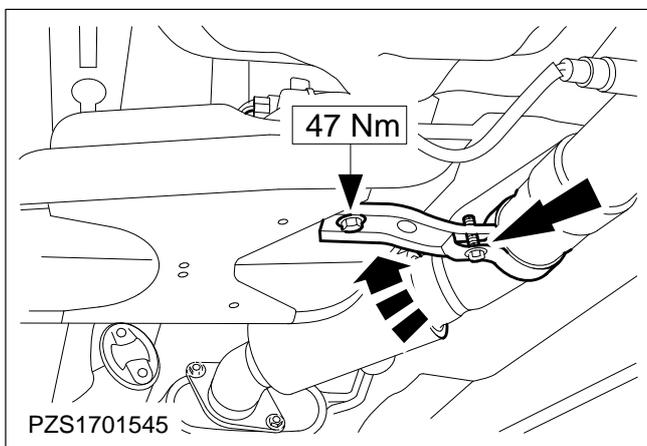
**13. Swivel the bracket for the front exhaust pipe upwards and attach it to the transmission crossmember.**
