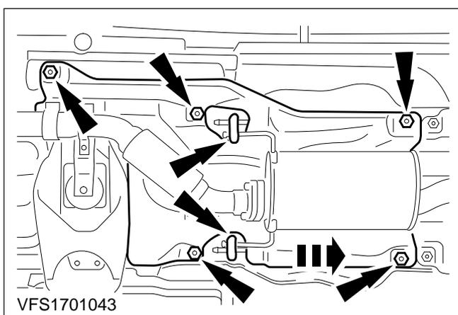
**14. Attach the front heat shield and hook the loops for the rear exhaust pipe in place.****15. Lower the vehicle.**
