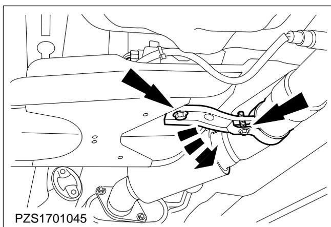
5. Detach the bracket for the front exhaust pipe from the transmission crossmember and swivel it downwards.
