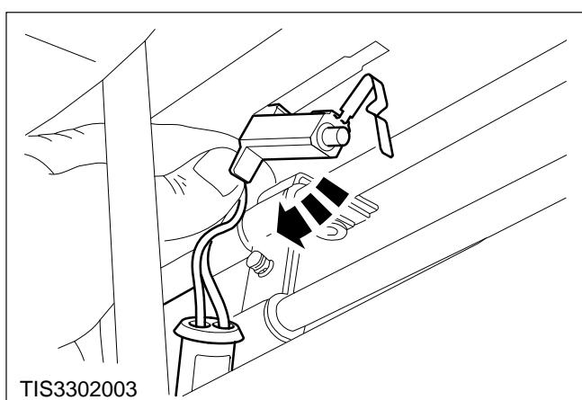
**3. Remove the low air temperature sender unit.**
