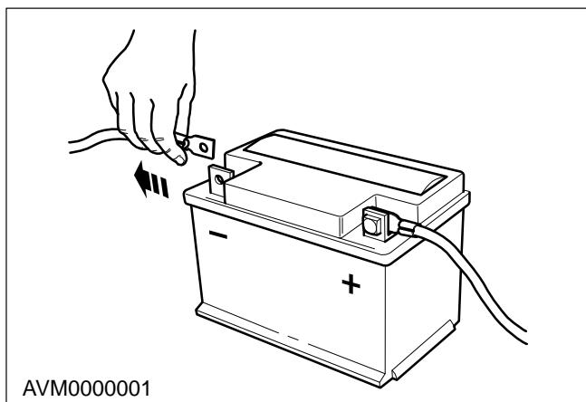
**Remove****1. Disconnect the battery negative lead.**
