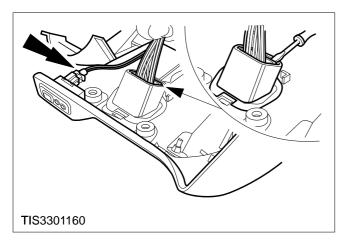
**NOTE:** There is no need to disconnect the hood release cable.
