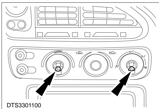
2. Remove the two screws retaining the heater control bezel.
