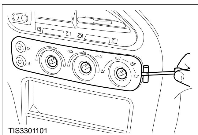
**CAUTION:** Only prise out the bezel from the air distribution control switch side of the bezel to prevent breakage of the locating tang at the opposite side.
