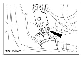
6. Remove the pinch bolt and nut securing the flexible coupling to the steering gear pinion shaft and remove the coupling.
