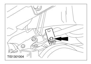
4. Remove the clamp plate bolt securing the flexible coupling to the steering column shaft.
