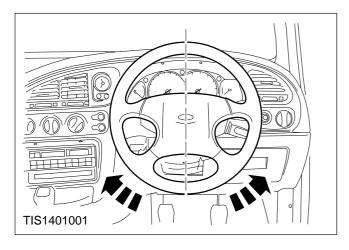
2. Centralise the steering wheel and lock in position.
