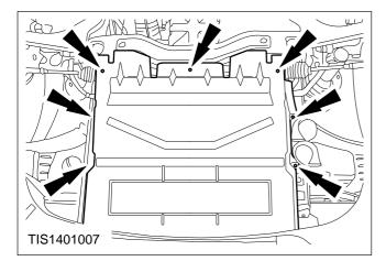
3. Raise the vehicle and remove the lower engine shield.
