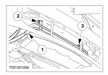
CAUTION: After removing the fluid cooler refit the fluid cooler retaining nut and bolt to hold the oil cooler in place.
