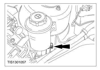
2. Disconnect the fluid cooler hose from the reservoir.
