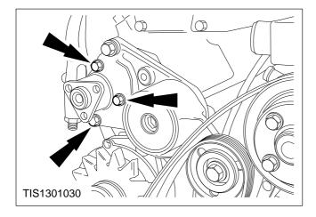
10. Remove the power steering pump.
