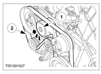
Belt – Power Steering – Pump Drive – Remove (13 424 0)
