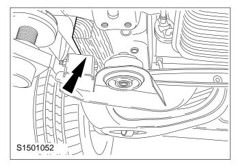
3. Place a wooden block between the floor assembly and the rear axle crossmember.
